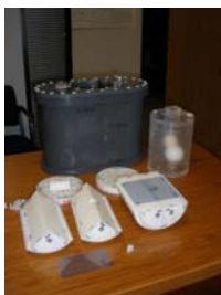
Figure 1: (left) The RPC Pelvis phantom with imaging insert and dosimetry insert. The dosimetry insert has been dismantled to show the film.
